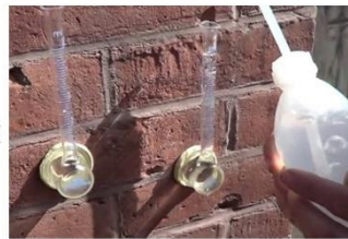
Inspect the Existing Masonry. Do masonry units need repair or replacement? Repointing required? How abundant is the brick? How, where there was a question about primary Karsten Tube testing is being done at random bricks and mortar joints.
