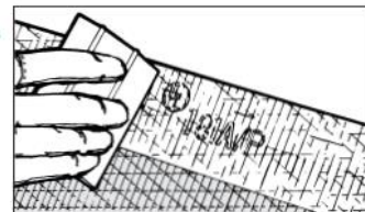
Fig. 4-3B. Rub tape firmly with plastic sealing tool until the facing reinforcement shows clearly through the tape. Avoid tearing or puncturing tape at staples.
