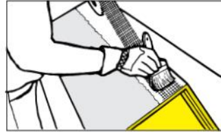
Fig. 4-5A. Apply a thin coat of mastic over the center of the joint seam. Embed glass fabric in mastic.
